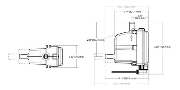
Typical mounting bracket installation and dimensions (4 possible orientations)
